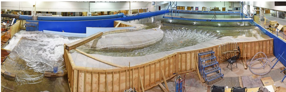
A panoramic photo shows the hydraulic model design for the U.S. Army Corps of Engineers Sacramento District's Isabella Lake Dam Safety Modification Project. The 1:45 scale model allows engineers to test the design against extreme storms and improve it before construction begins. U.S. Army Corps of Engineers via Flickr.
