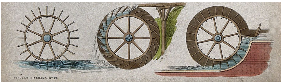
Illustrated diagram showing an undershot waterwheel (left), overshot waterwheel (middle), and breastshot waterwheel (right)
